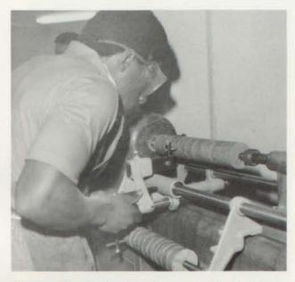
Clayton Brooks is using the new lathe duplicator — a machine that simplifies the making of identical parts on the wood lathe.
